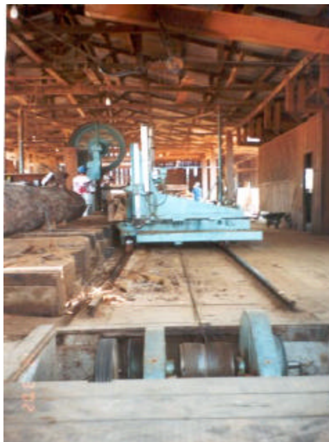
Traction for wagon introducing log to bandsaw
