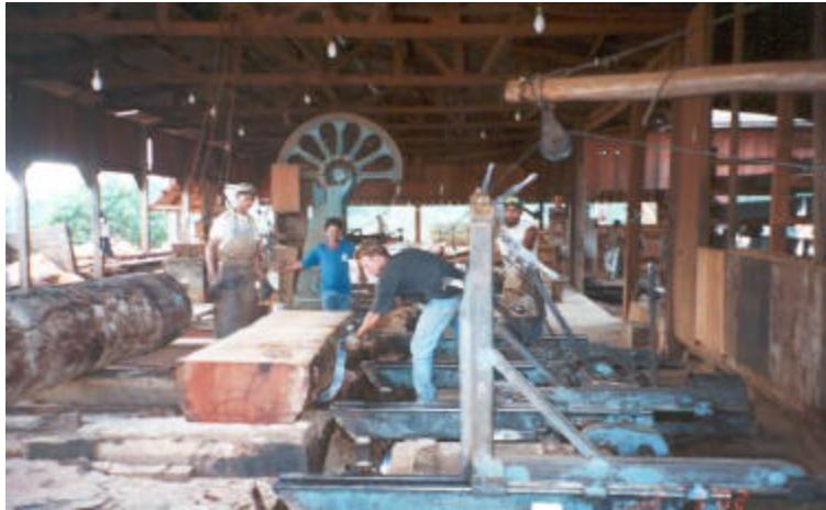
Repositioning partially cut log for bandsaw
