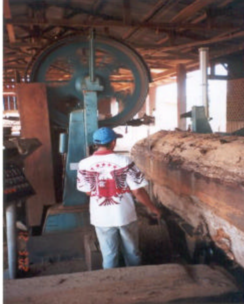
Introducing the log to the bandsaw
