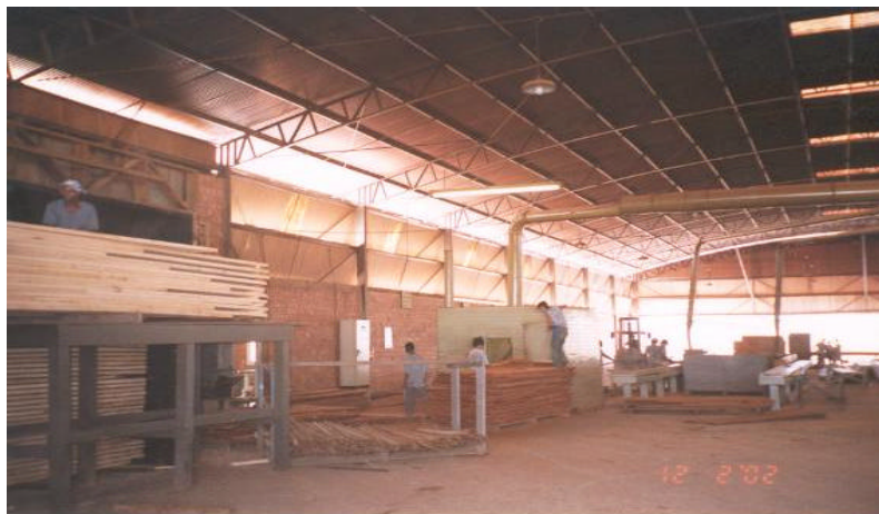
Product finishing line in shed with driers
